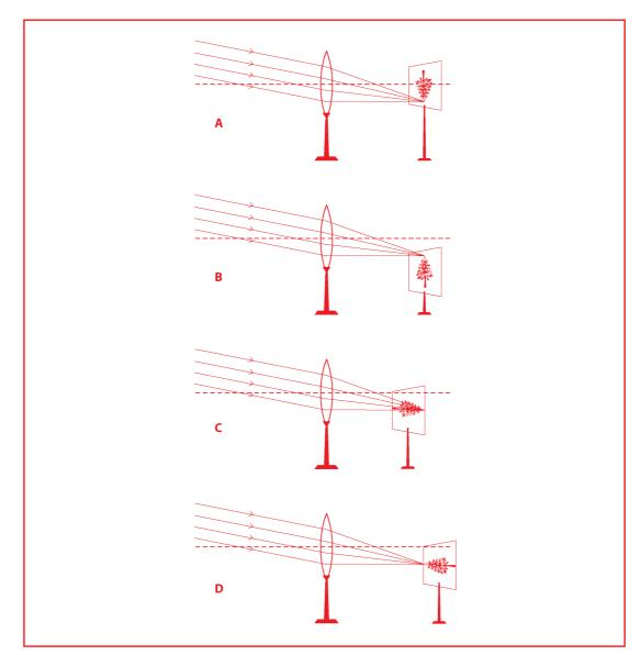
15. Parallel rays a distant tree incident on a convex lens form an image of the screen.
