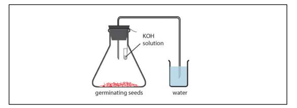
In this set up, the small test tube containing pellets of KOH is kept in the conical flask to absorb
